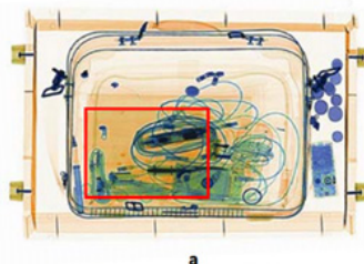
Figure 2: The bag of Figure 1 scanned with a multi-view imaging system with automated explosives detection (EDSCB). a) Main view b) Side view. Red frames indicate areas in the bag that might contain explosive material.
