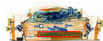
Figure 2: The bag of Figure 1 scanned with a multi-view imaging system with automated explosives detection (EDSCB). a) Main view b) Side view. Red frames indicate areas in the bag that might contain explosive material.
