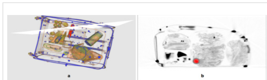
Figure 3: A bag scanned with a 3D imaging system for CBS. a) 3D rotatable image b) Cross-sectional image. Red color indicates areas in the bag that might contain explosives. Images are from a 3D training simulator for CBS (X-Ray Tutor Version 4 [XRT4]) provided by CASRA.
