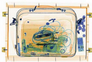
Figure 1: Conventional single-view X-ray image of a cabin bag (from [6]).
